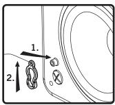
**8.** Attach grille safety clip by placing the large end of the clip over snap-fit post (1), then sliding clip until small end snaps into place around post (2).
